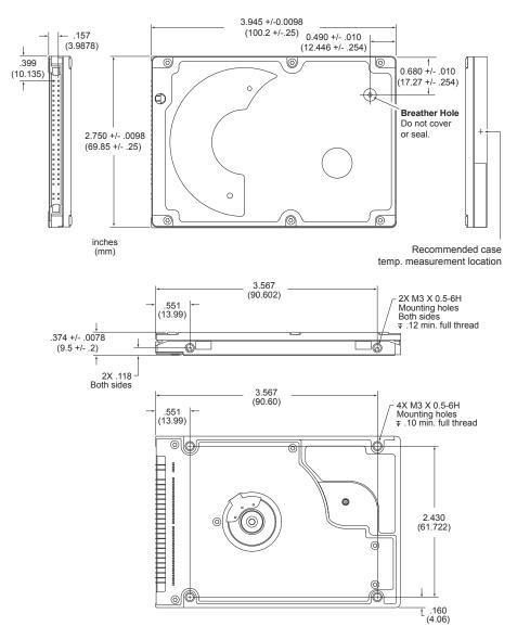
Figure 4. Mounting dimensions-top, side and end view
